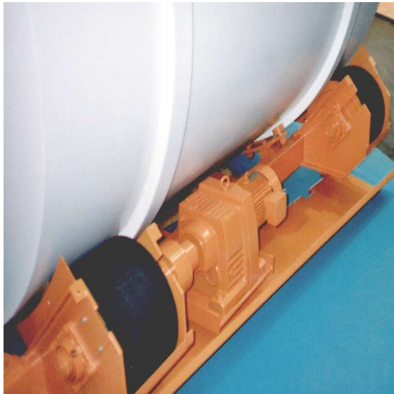
detail: dewatering drum drive
