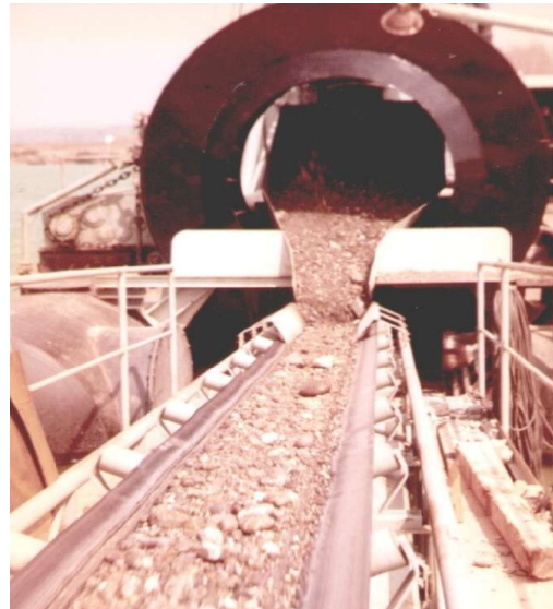
aggregate after dewatering, 350 t/h
