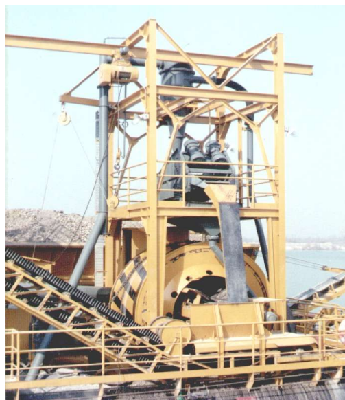
Pressair dewatering drum 400 t/h with optional cyclone/screen system
